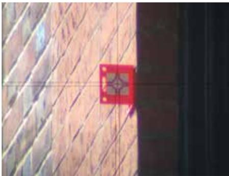
Figure 3. Collimation of a target through a total station.
