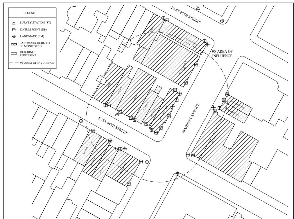
Figure 2. Monitoring plan diagram with 90 foot radius indicated.
