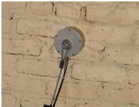
*Figure 7. Attachment of a vibration monitor geophone.*
